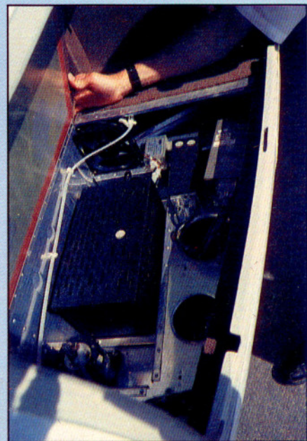
Cessna attempted to minimize the Crusader's operating costs by providing easy access for maintaining components. The cabin heater and several black boxes, for example, are located beneath the front baggage compartment.
