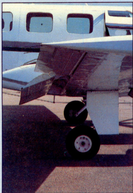
Trailing-beam main gear makes landings simple and pleasant. Strakes mounted next to the wing roots (right) and on the engine nacelles improve airflow separation characteristics and smooth the flow of air over the elevator.
